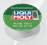
Special cord made of high-strength, plaited polyethylene fibers. For separating windows which are located very low on the body flange, e.g. for newer Audi and Volkswagen models. The tiny diameter of 0.5 mm allows you to pull the cord manually – or you use the LIQUI MOLY Glass Pane Separator (part no. 7944).
