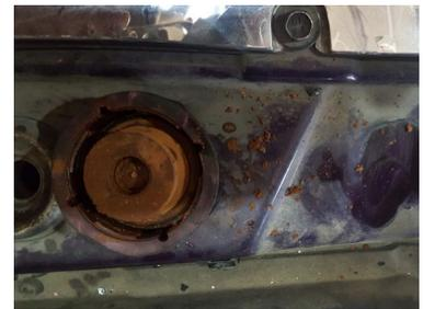
Corrosion deposits in the compensating reservoir and in the cap.
