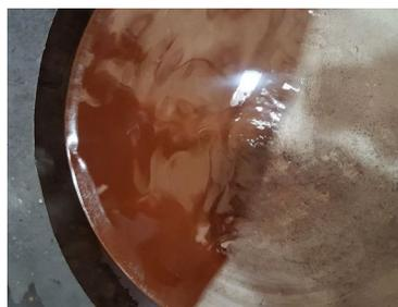
Corrosion deposits in the coolant. Such contamination proves that the entire cooling system is affected by corrosion.
