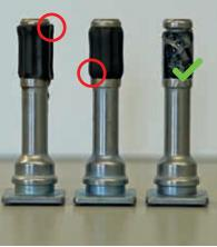
The illustration provides a striking example of what happens if the wrong grease is used. The rubber component swells up, reducing the braking power and causing the brake to seize.
