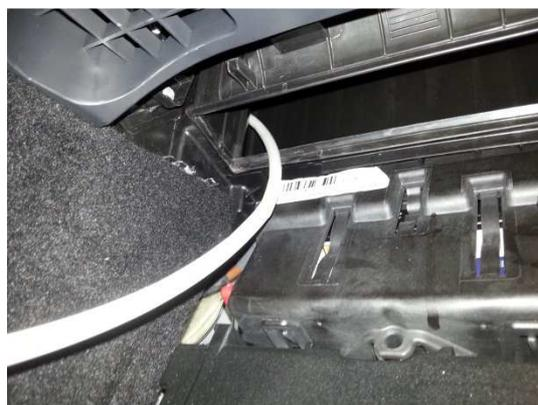
8. Activate the cleaning gun and sweep the probe back and forth across the evaporator using approx. 0.9 litres of the LIQUI MOLY AIR CONDITION CLEANER.
