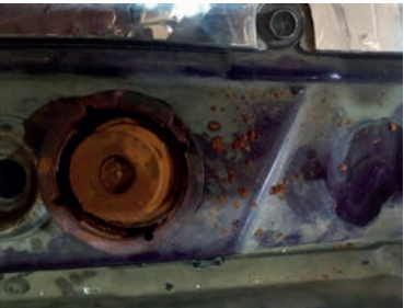
Corrosion sediment in the expansion tank and lock.
