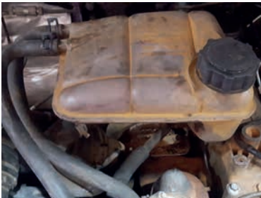
Corrosion sediment in the expansion tank and lock.
